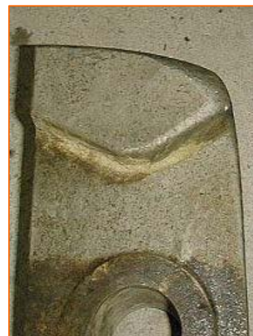
In fig. No.2 Mn Steel hammer after 2500working Hours.
