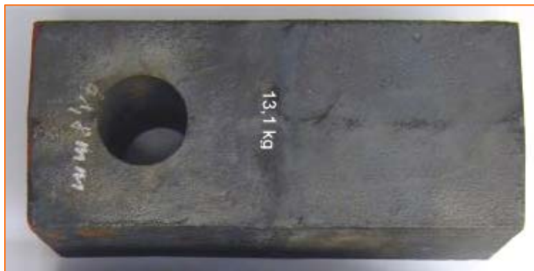
In fig. no. 1 this is the typical Clinker Crusher Hammer made of MN Steel III has used to crush clinker.
