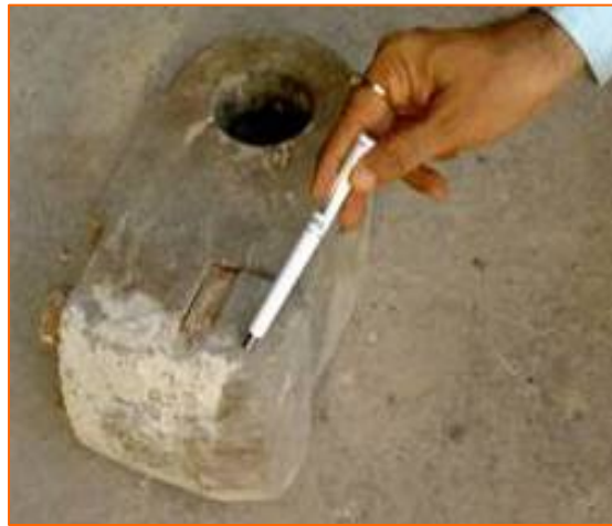
Fig. no. 5 linker Crusher Hammer with Zuper Block Replaceable Carbide tip
