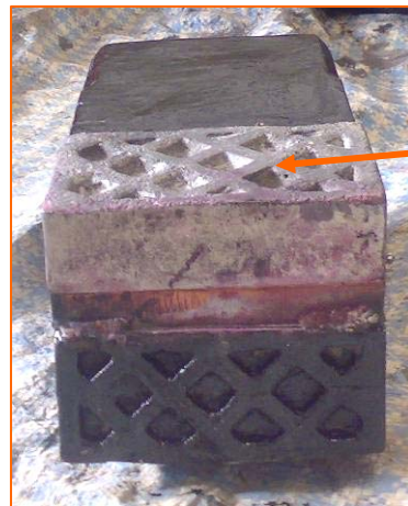
Fig. No. 4 - Clinker Crusher Hammer Body with Zuper Replaceable Block Carbide tip
