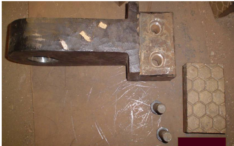
Fig. No. 3 - Clinker Crusher Hammer Body & Zuper Replaceable Block Carbide tip
