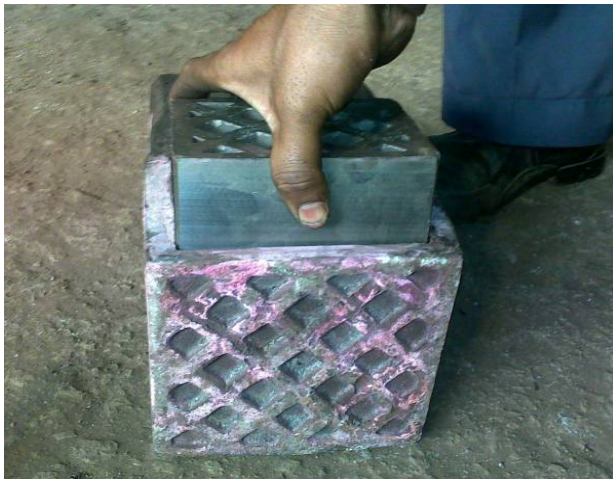
Fig. 3 & 4 - Zuper Block composite sintered carbide assembled with Clinker Crusher Hammer & tighten the bolt with Torque Wrench.
