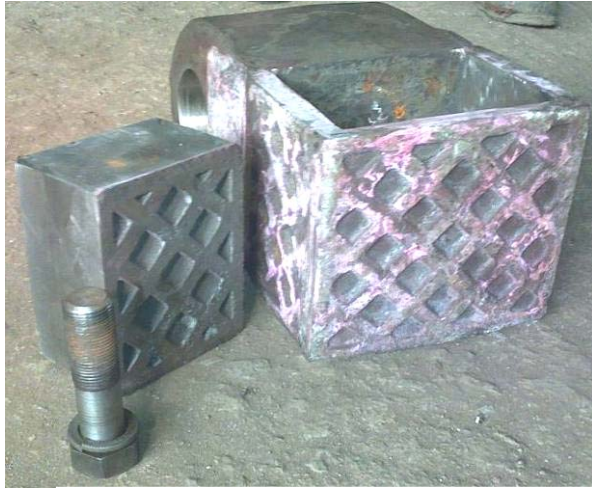
Fig. 1 & 2 – Assembly of Clinker Crusher Hammer with Zuper Block Sintered Composite Carbide
