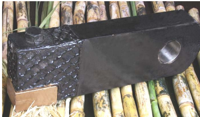
Fig. No. 3 – Swing type Fibrizor Hammer Body with Zuper Replaceable Block Carbide tip
