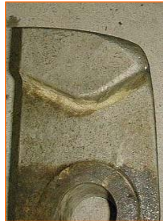
Fig. No.2 - Mn Steel hammer after 4500working Hours.
